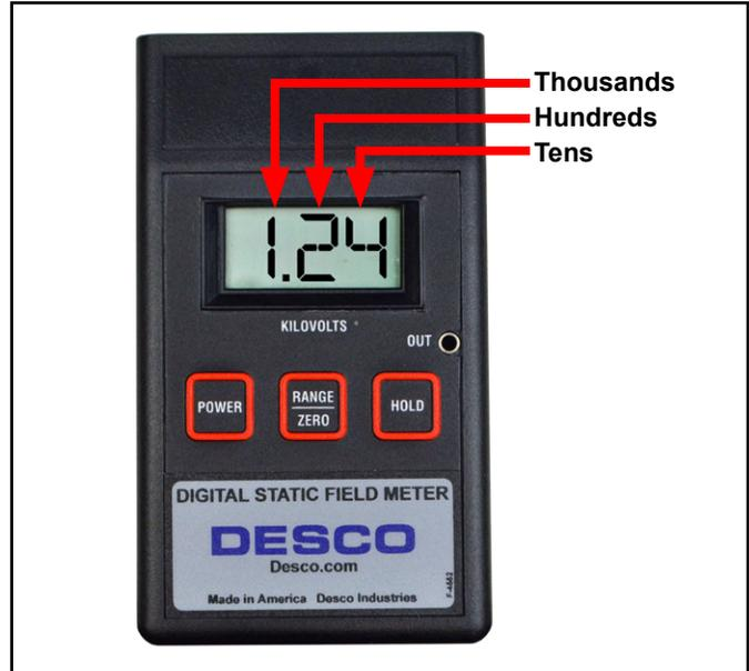
Figure 4. Reading the Digital Static Field Meter while in the  $\pm 20\text{kV}$  range
