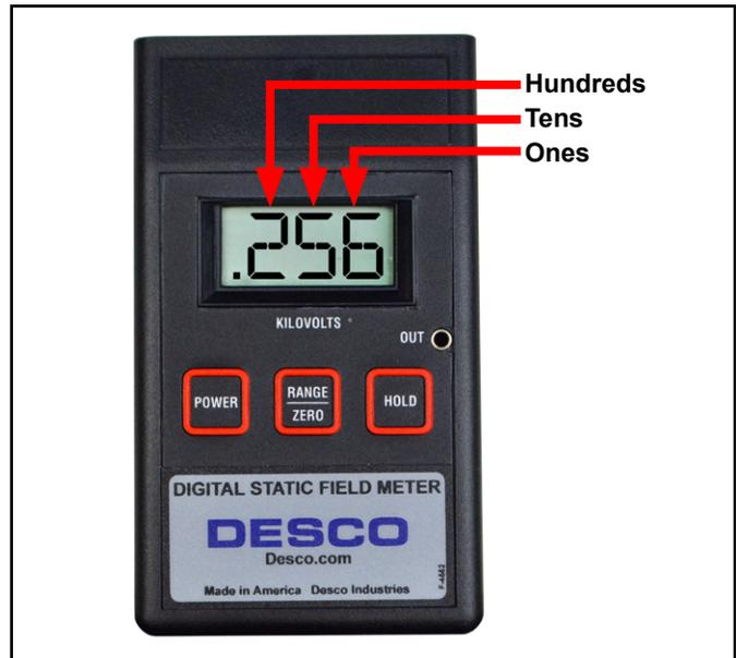
Figure 5. Reading the Digital Static Field Meter while in the  $\pm 2\text{kV}$  range
