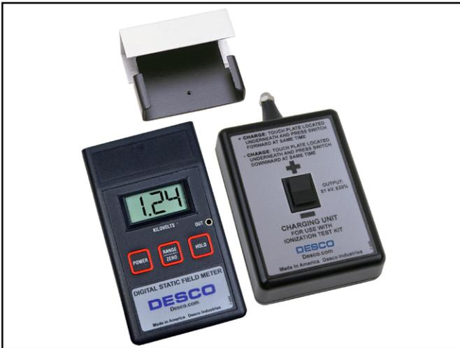
Figure 1. Desco [19493](#) Ionisation Test Kit
