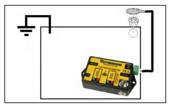
Figure 4. Installation method #2 of the Multi-Mount Continuous Monitor
