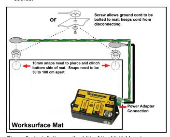
Figure 3. Installation method #1 of the Multi-Mount Continuous Monitor
