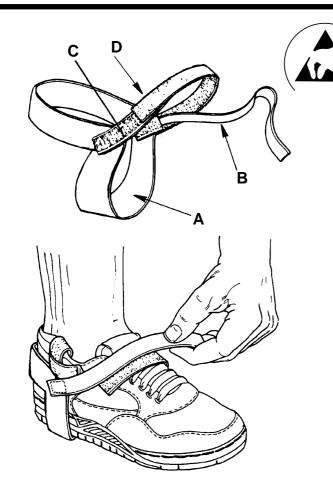
**Caution:** The foot grounder is for ESD control. It will not reduce or increase your risk of receiving electric shock when using or working on electrical equipment.
